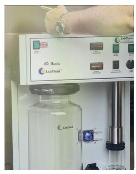
Ensure the glassware and accessories are fitted to the SD-Basic, with your sample solution ready, before turning the compressor on, setting between 1-3 Bar.
