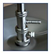
The assembly incorporates an automatic de-blocking device that prevents the jet nozzle from becoming blocked, the de-blocking needle is activated by an integral compressor.
